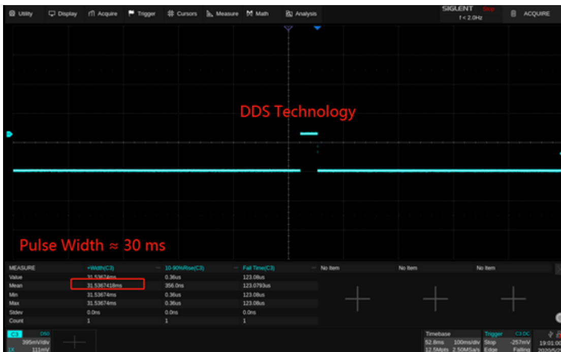
Figure 6: 1 Hz pulse signal generated by DDS
