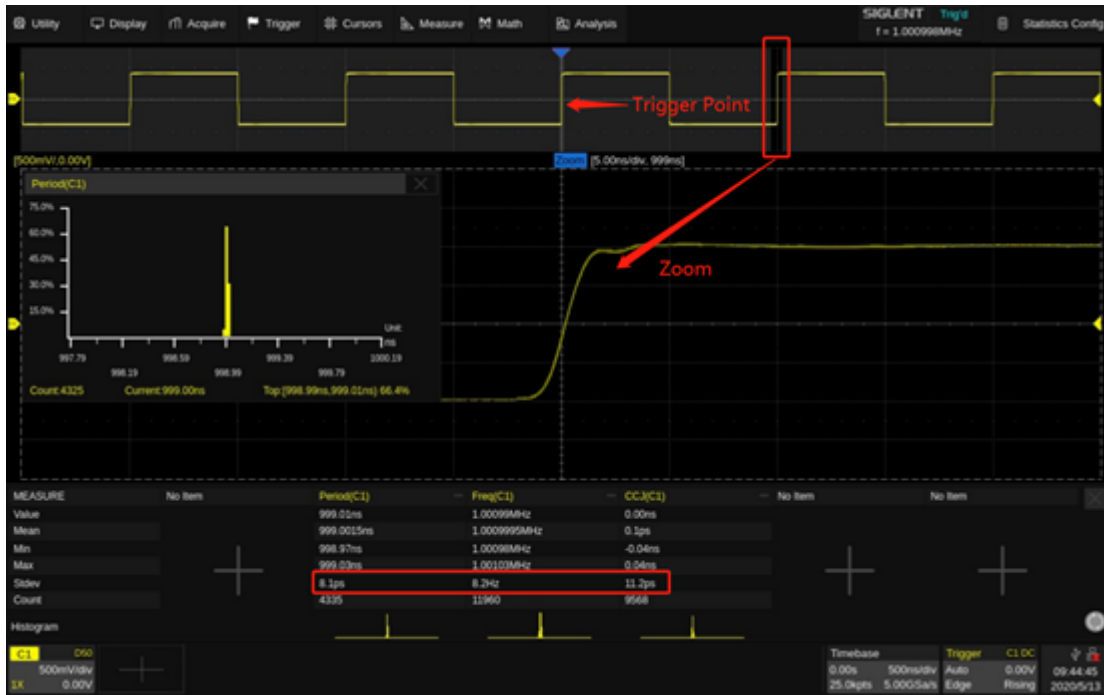
Figure 5: EasyPulse waveform with low jitter
