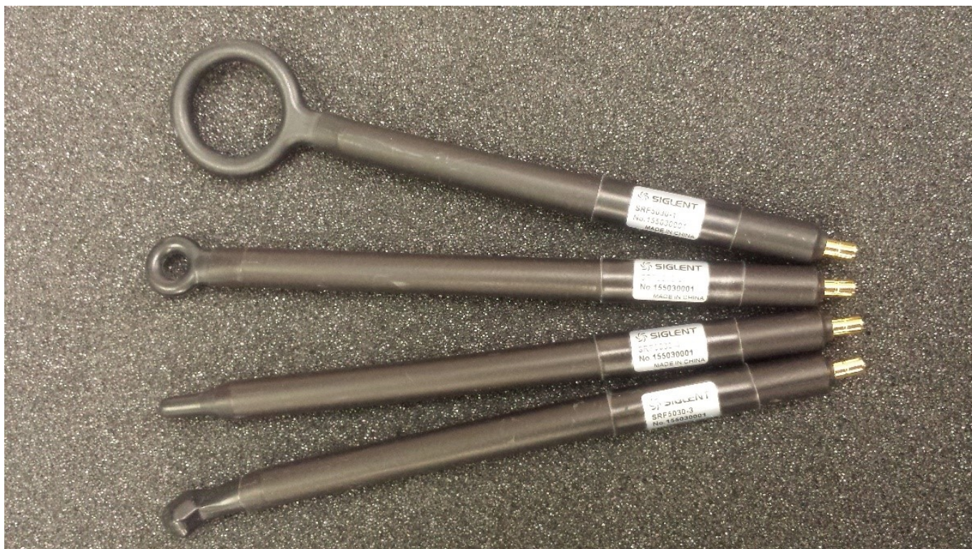
Figure 3: Siglent SRF5030 Near-Field Probe kit includes 2 loop and 2 point magnetic (H) field probes, cable, and adapter. Only the probes are shown.
