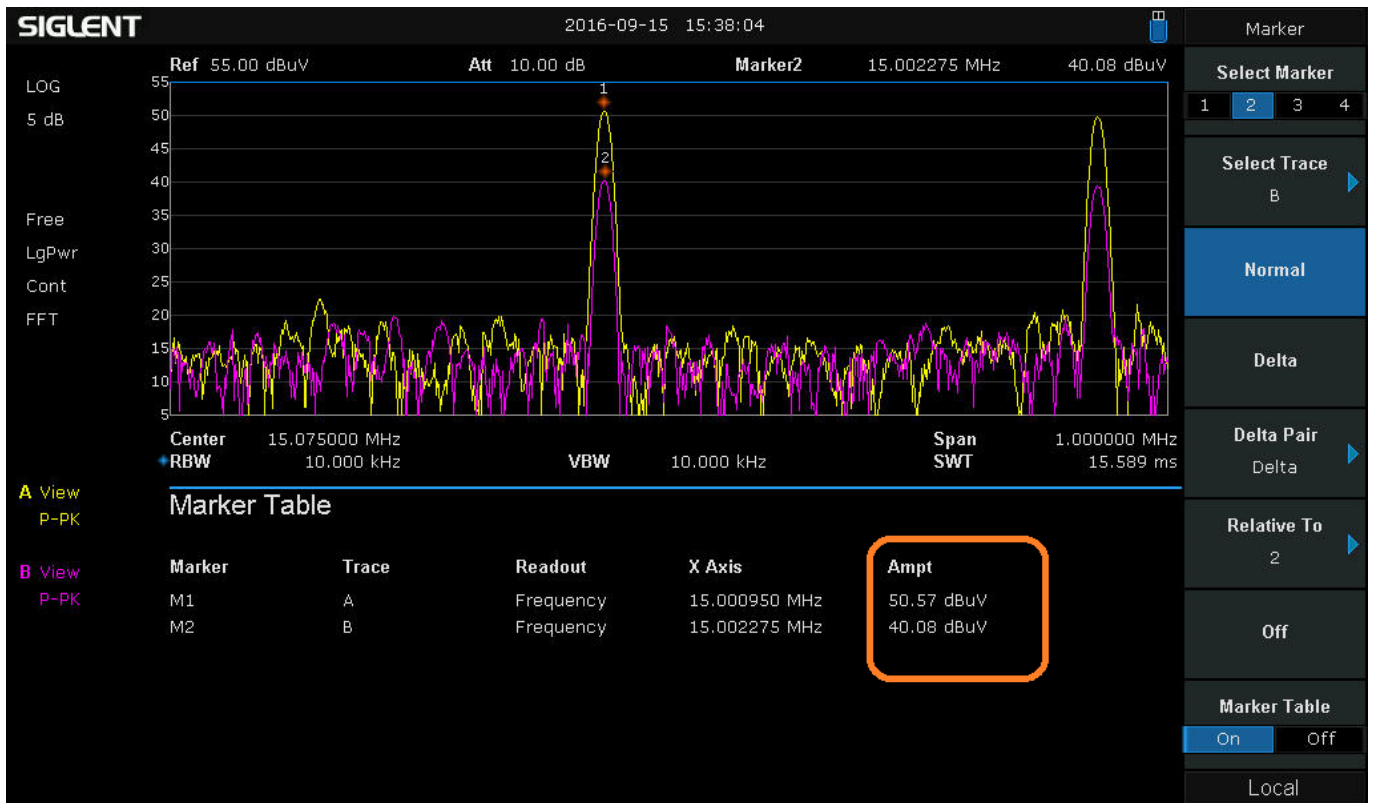
Figure 10: Comparison of two scans using the marker table function of the SIGLENT SSA3000X spectrum analyzer. The Yellow trace was collected without attenuation while the Pink trace was collected after adding a 10 dB external attenuator.
