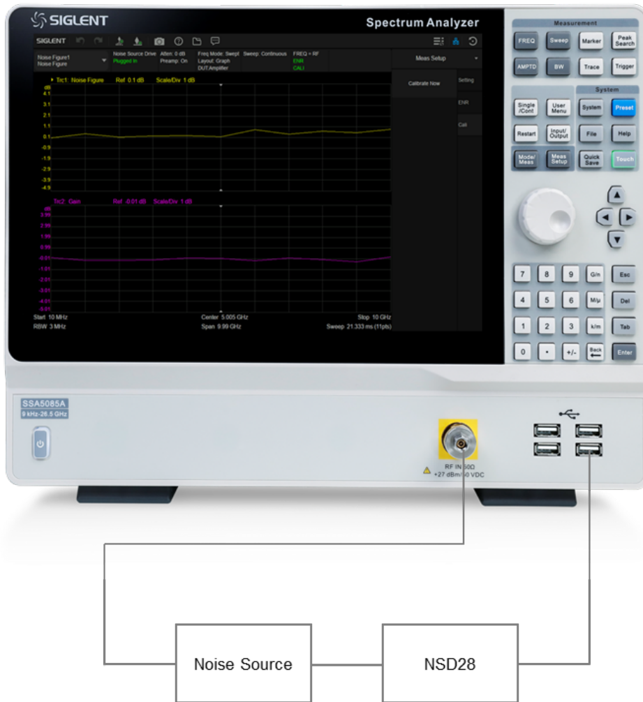
Figure 1-2 Connection setting of noise figure measurement calibration
