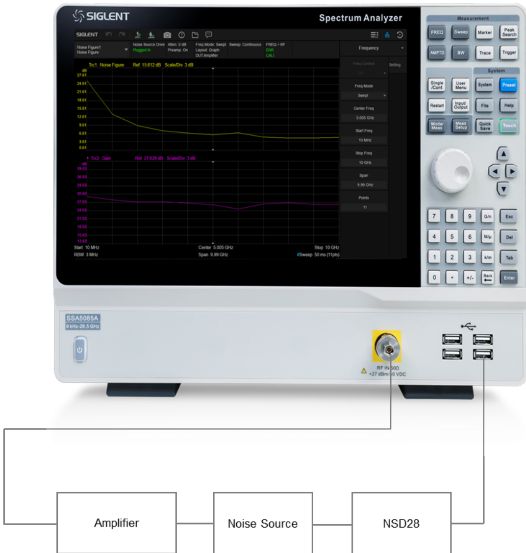
Figure 1-6 Connection settings for noise figure measurement
