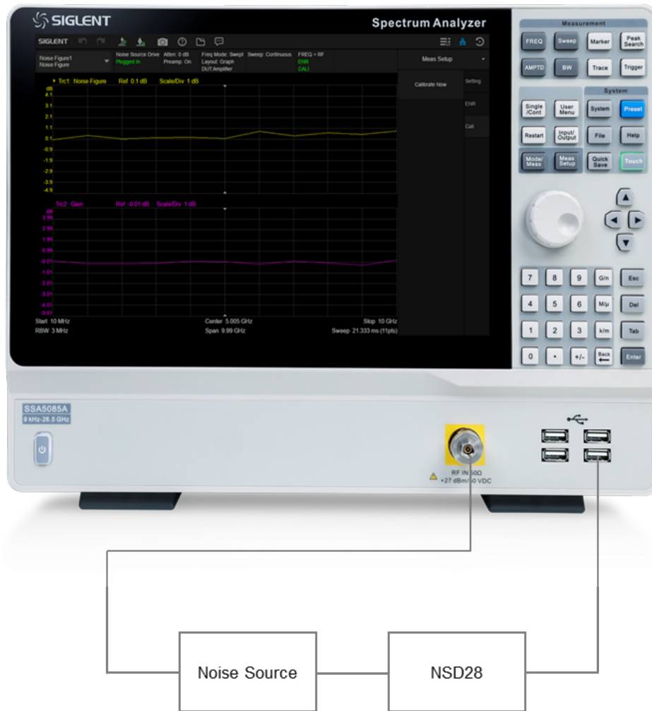
Figure 1-2 Connection setting of noise figure measurement calibration
