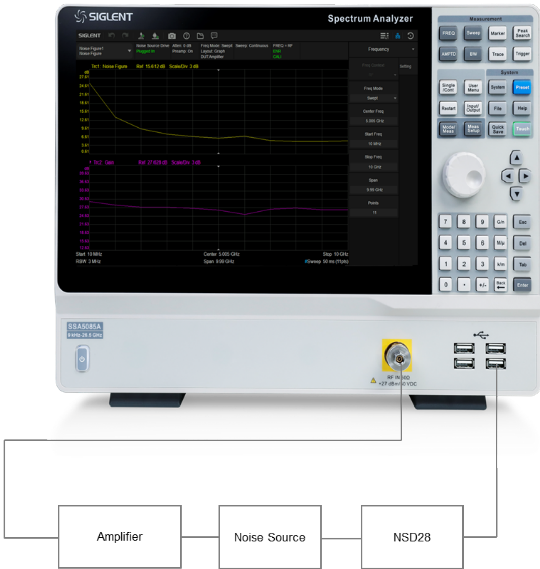
Figure 1-6 Connection settings for noise figure measurement
