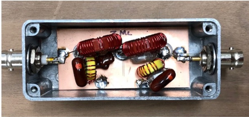
3rd Order Inverse Chebyshev Bandpass Lower Cutoff Freq. = 2.750 MHz; Upper Cutoff Freq. = 3.250 MHz Passband Attenuation = 50.0 dB
