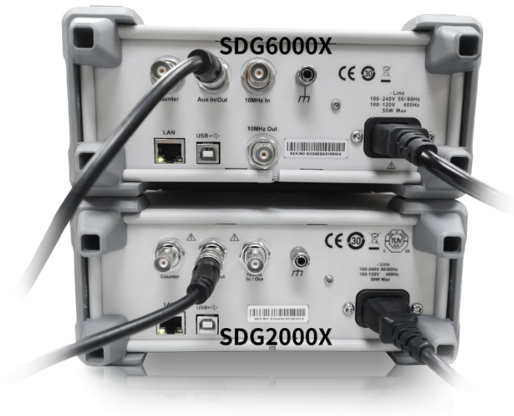
Figure 2. Connect SDG2000X and SDG6000X Aux In/Out
