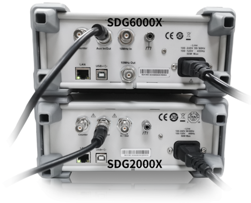
Figure 2. Connect SDG2000X and SDG6000X Aux In/Out
