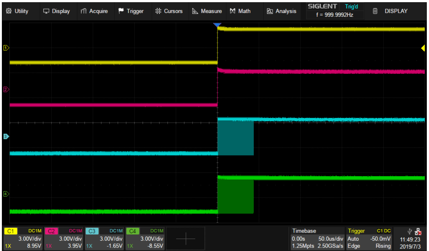
Figure 4. Four signals phase drift without synchronization
