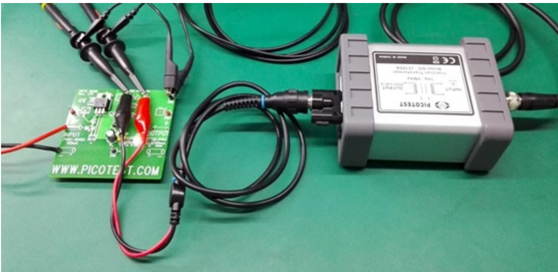
Figure 9: Probe and Transformer connections to the DUT
