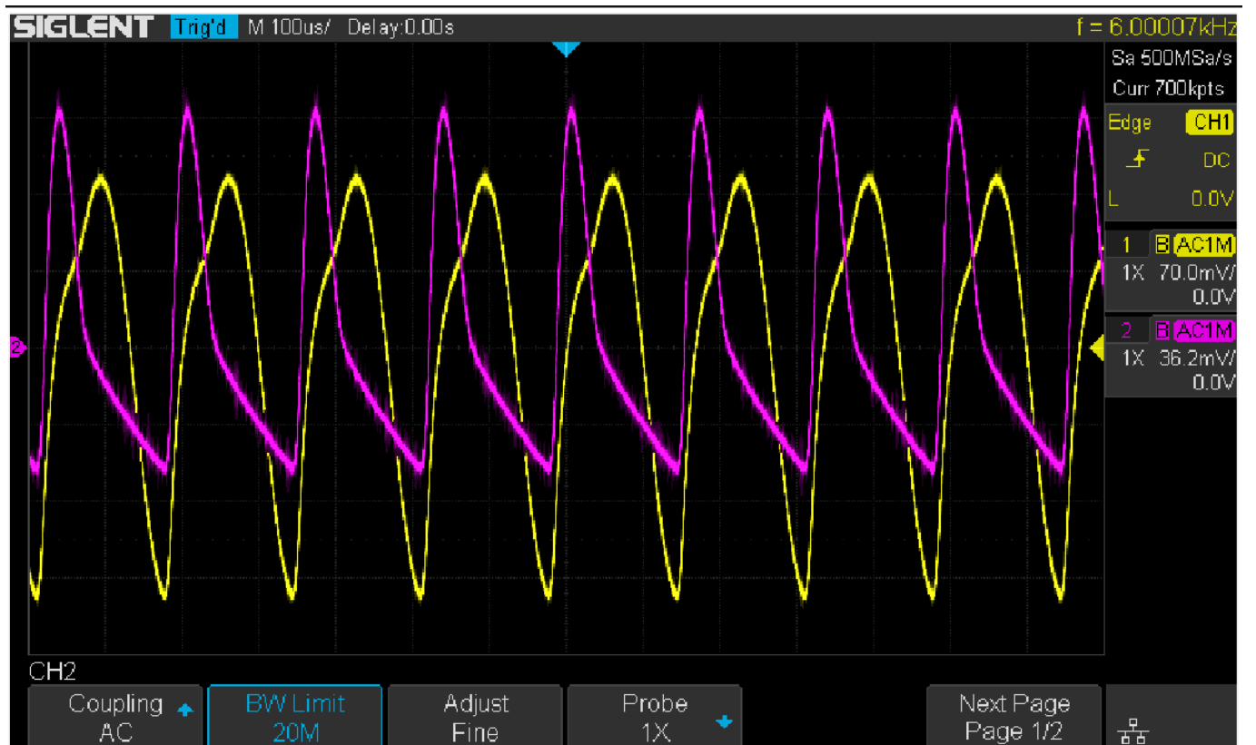
Figure 15: Distortion in the time domain
