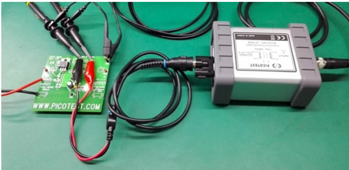
Figure 9: Probe and Transformer connections to the DUT
