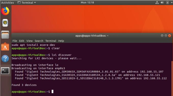
Here, we have three devices connected: an SDM3065X, SSA3032X, and an SDS1102X-E (which has been superseded by the SDS1202X-E series here in North America). It also includes the instrument serial number, firmware revision, and IP address.
