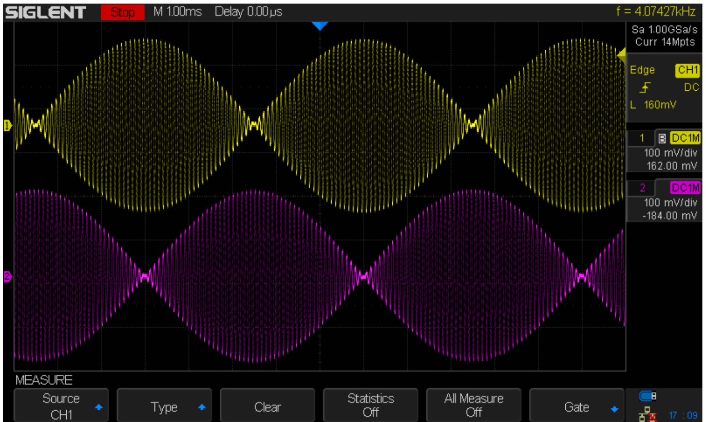
Figure 6: Primary coil 10 kHz, secondary coils at 100 Hz.
