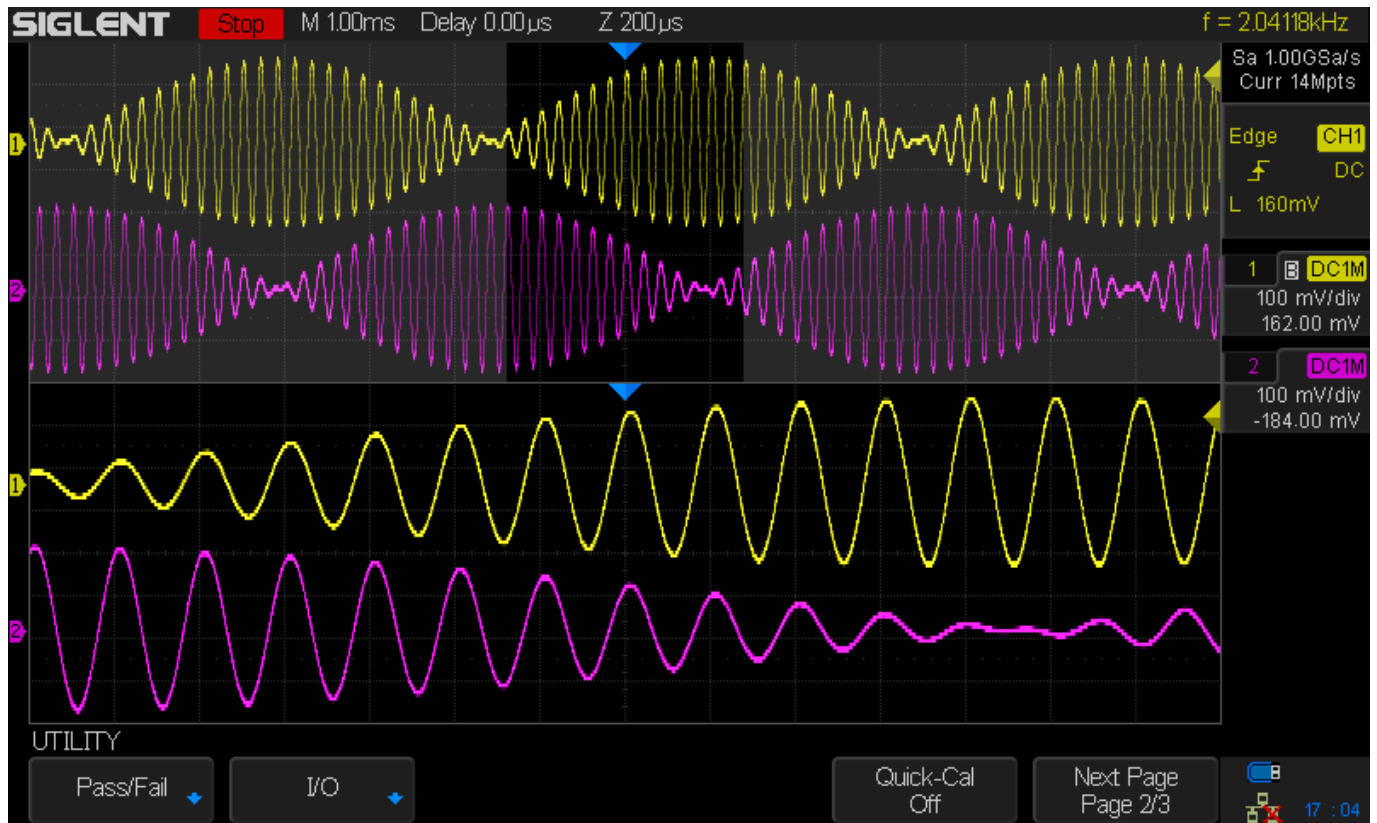
Figure 9: Primary modulation voltage is correct. Note the smooth edges of the waveforms.
