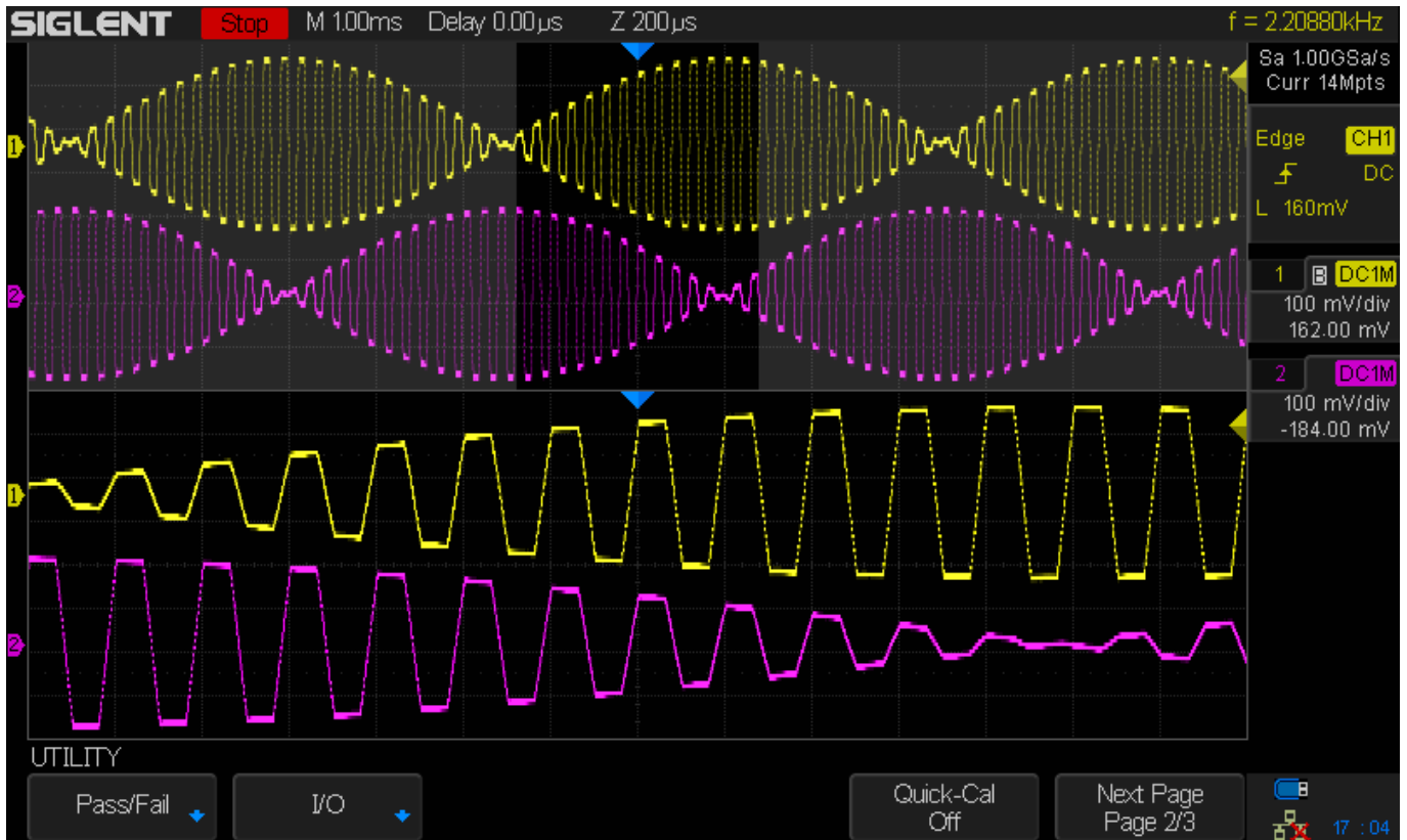
Figure 8: Primary modulation voltage is too high. Note square edges of the waveforms.
