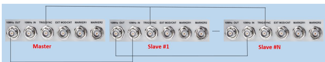
Figure 17-1 wiring diagram of multi-device synchronization
