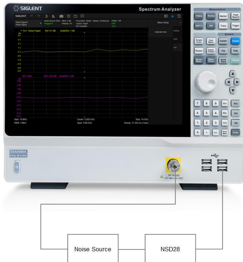
Figure 1-2 Connection setting of noise figure measurement calibration
