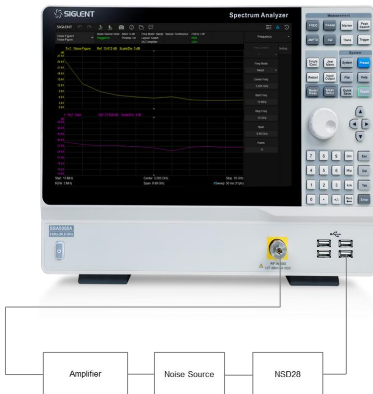
Figure 1-6 Connection settings for noise figure measurement
