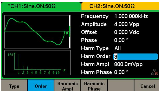
Up to 16 harmonics may be generated. Amplitude and phase of each harmonic can be set independently
