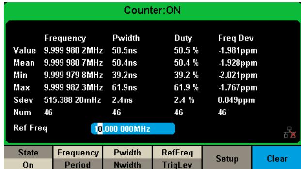
High precision Frequency Counter with an input frequency range of 0.1 Hz~200 MHz.
