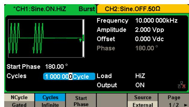
Two Burst modes, "N cycle" and "Gated". The Burst source can be configured as "Internal", "External" or "Manual".
