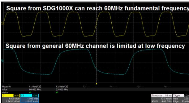
Benefiting from a special square-wave generating circuitry, the Square from the SDG1000X breaks the 60 MHz bandwidth barrier, reaching rise/fall times of less than 4.2 ns, and frequencies up to 60 MHz.
