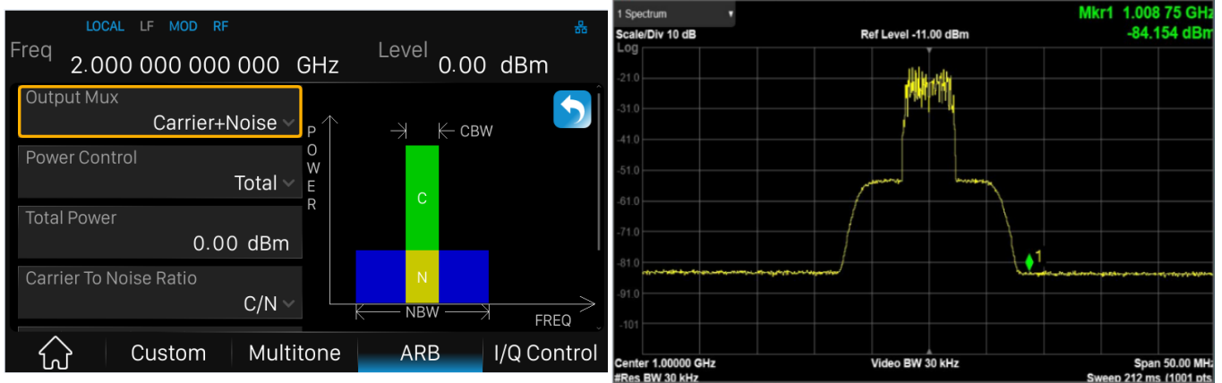
Add real time AWGN to digital IQ signals for receiver performance tests
