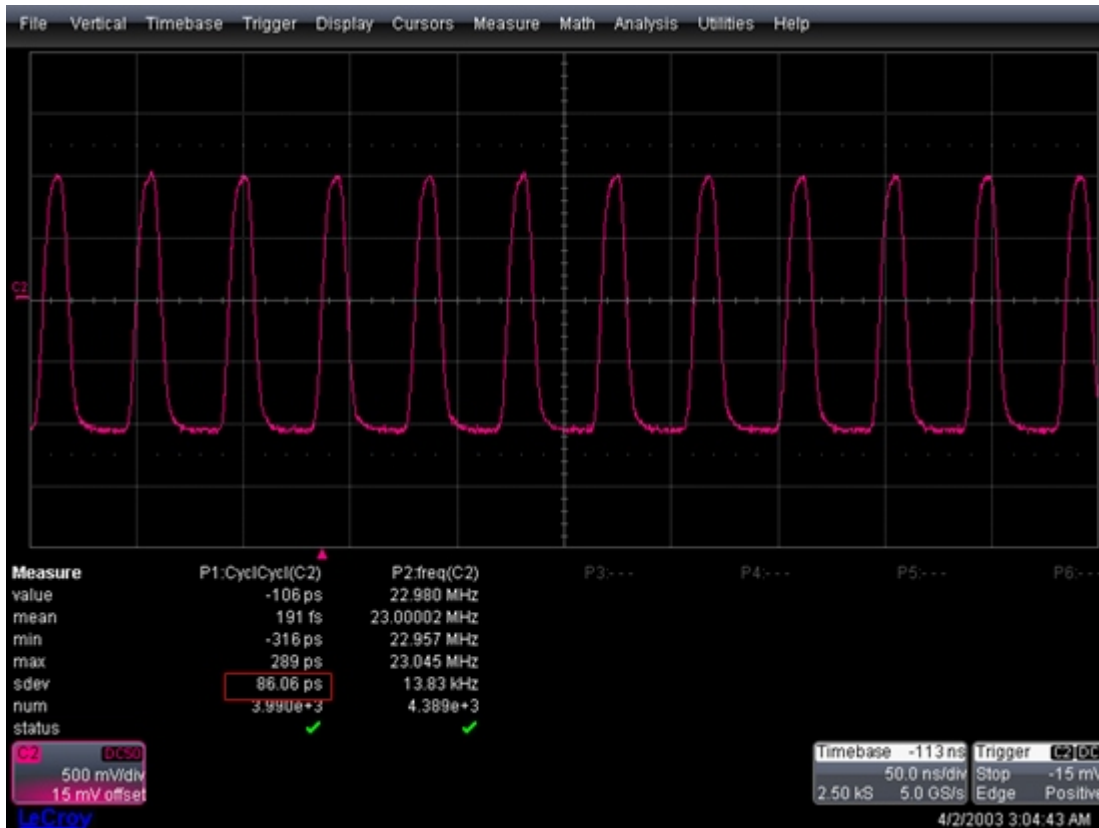
P4 EasyPulse waveform with low jitter
