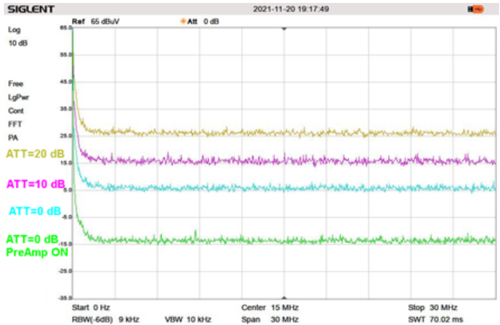
Figure 8: DANL versus internal attenuator / pre-amplifier settings. RF input terminated with 50 Ohm.
